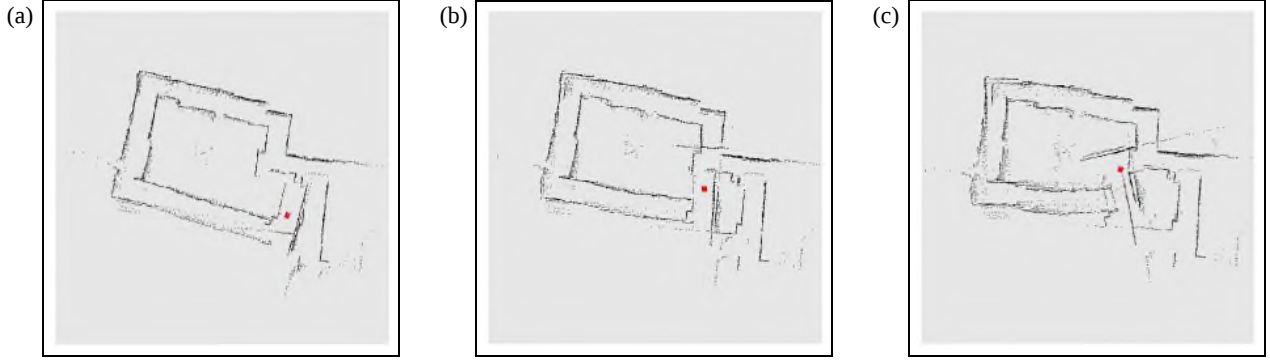
Figure 6: Incremental maximum likelihood mapping: At every time step, the map is grown by finding the most likely continuation. This non-probabilistic approach works well in non-cyclic environment but is generally unable to handle cycles.
